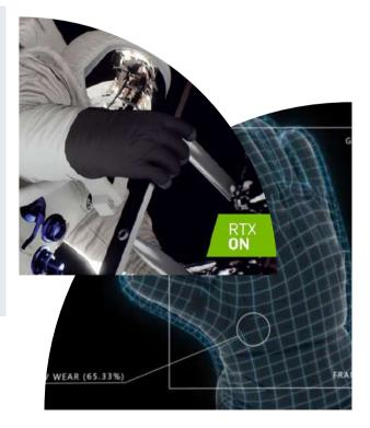
To create the glove analyser, the project's team first started with images of new, undamaged gloves and those which featured wear and tear from spacewalk and terrestrial training. NASA engineers went through the images and tagged specific types of wear through Azure Cognitive Services' Custom Vision.
